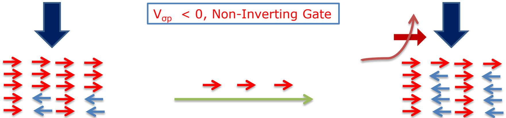
The dominant magnet injects net spin into the output forcing output to align
