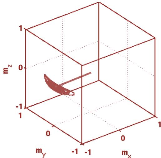
Origin of the magnetic retention/write/read failure is thermal noise which continuously perturbs the magnet's internal field.
