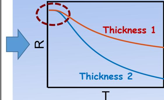
Thickness *independent*  $R_{xx}$  at low T plateau of bulk crystals
