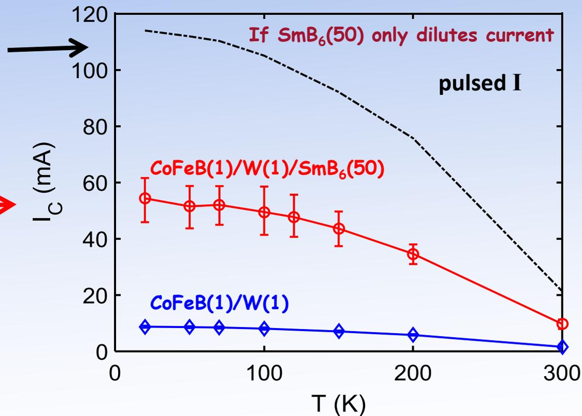
**$\text{SmB}_6$  reduces current for switching PMA layer**
